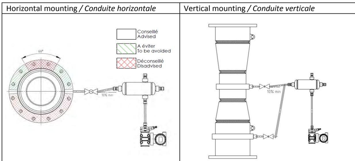
Fig 7 : Transmitter mounting for steam applications
