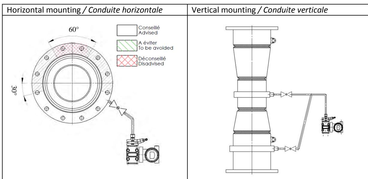
Fig 5 : Transmitter mounting for liquid applications
