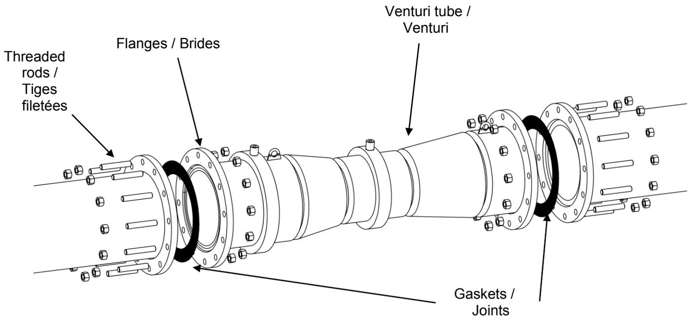
Fig 3 : Assembly of the venturi between flanges
