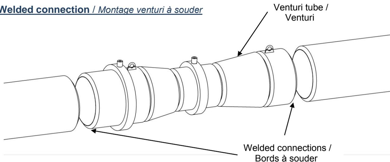
Fig 4 : Assembly of the venturi with welded connections
