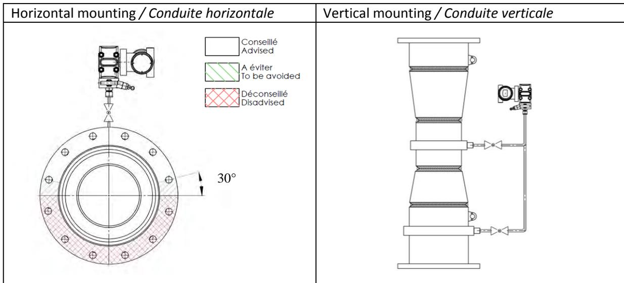
Fig 6 : Transmitter mounting for gas applications
