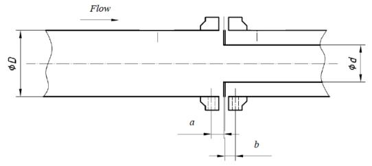
$a = b = (25, 4 \pm 0, 5)$  mm for  $\beta > 0,6$  and D < 150 mm  $(25, 4 \pm 1)$  mm for  $\beta \leq 0,6$   $(25, 4 \pm 1)$  mm for  $\beta > 0,6$  and 150 mm  $\leq D \leq 1$  000 mm
