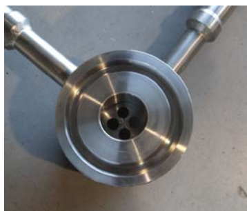
Picture 2 : 4 holes RTJ monoblock system with 2 nipples, pressure taps centered between 2 of the 4 bores
