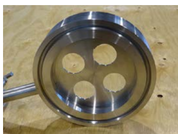
Picture 5 : 4 holes RTJ compact flowmeter (2 integrated pressure taps)
