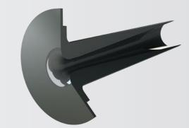
Sonic condition through the nozzle means that the flow reaches the velocity of sound when passing through the throat. Under these conditions, the flow rate depends mainly on the upstream pressure and the fluid temperature. This allows to deliver a steady and perfectly known flow rate, independent of the downstream pressure conditions from the nozzle.
